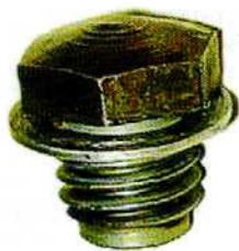
BELOW Owners of later Triumph and BSA twins and singles find a MIG diffuser makes a fine union for the timing plug.
